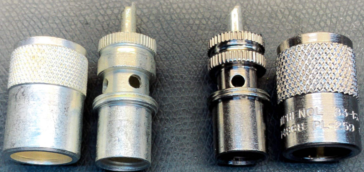
Nickel-plated PL-259 connectors, like the one at right, can be difficult to solder to. Silver-type connectors, like the one at left, accept solder more readily.
